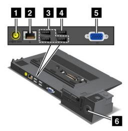
**1** Power jack: Connect the ac power adapter.
